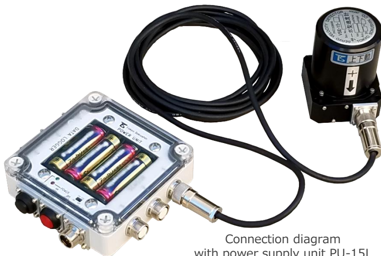
VSE-15L1 x 3-axis driven by external power supply (⇒ Power is 1/20 of the data logger and can be almost ignored)
